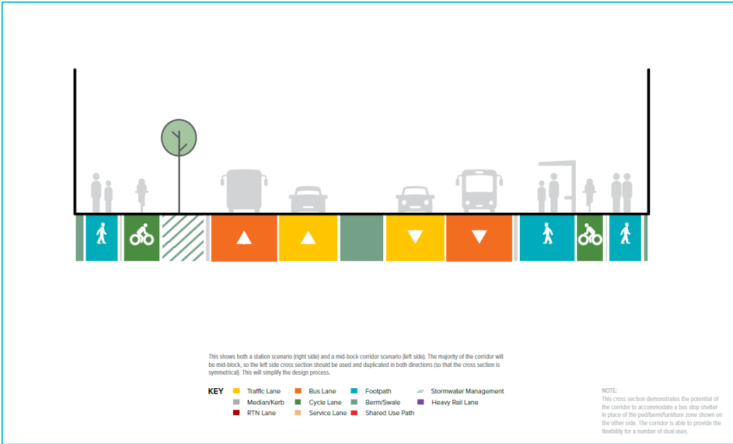
Figure 9-4 Indicative generic Four-Lane Arterial - 30m cross section with 2 lanes for general traffic, PT and active transport facilities either side. Proposed SH22 to Burt Road (not to scale)
