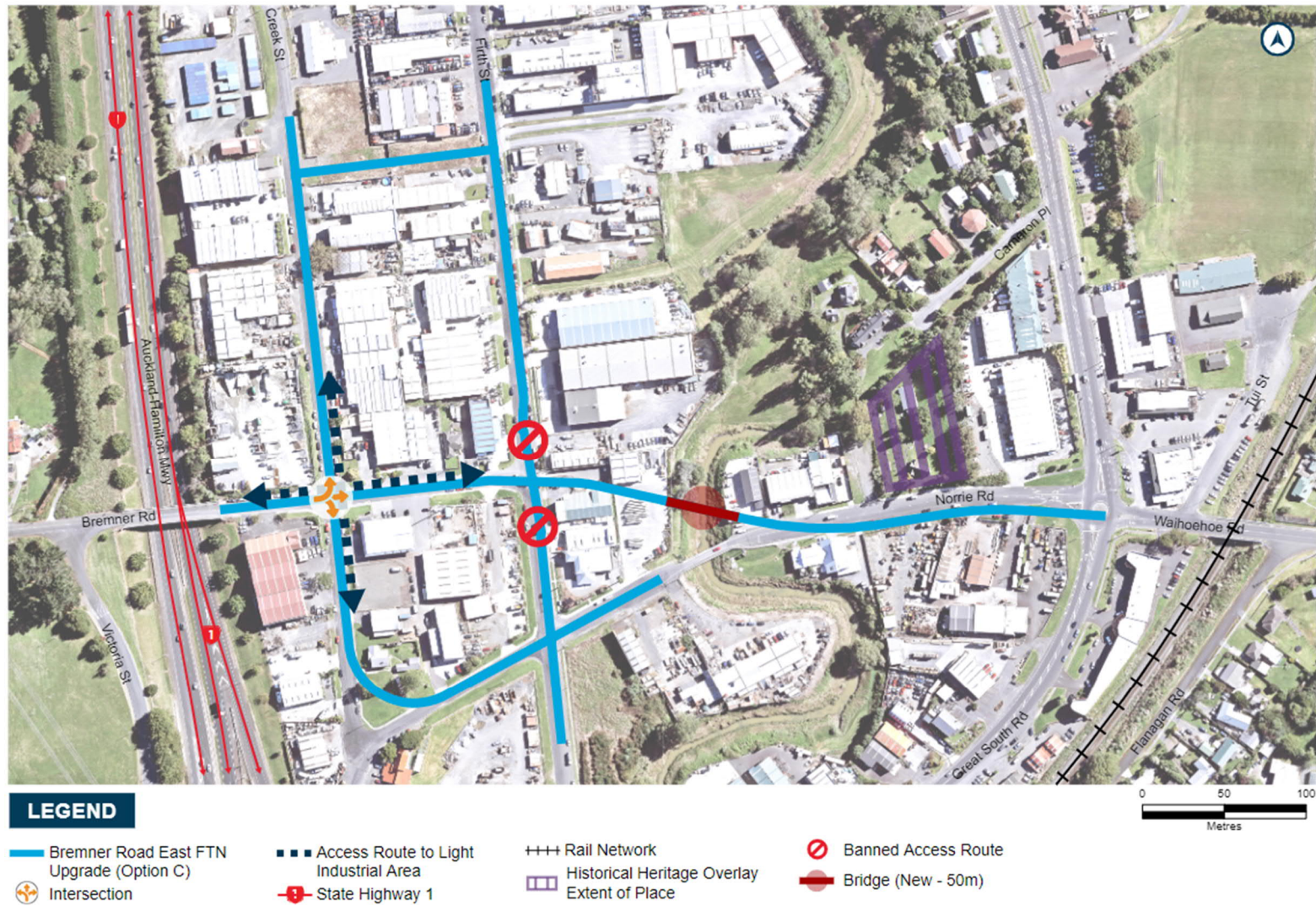
Figure 11-14: Option C – short bridge, Fifth Street rerouted
