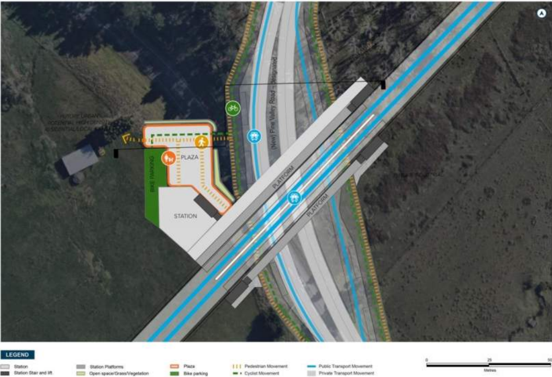
Figure 69: Indicative Pine Valley East Station Design
