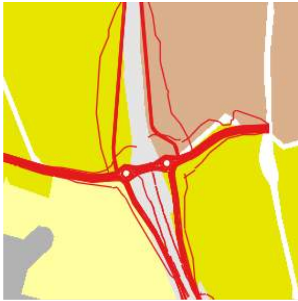
Option C: W42_SH-12 (Wilks Road interchange south with loop onramp)
