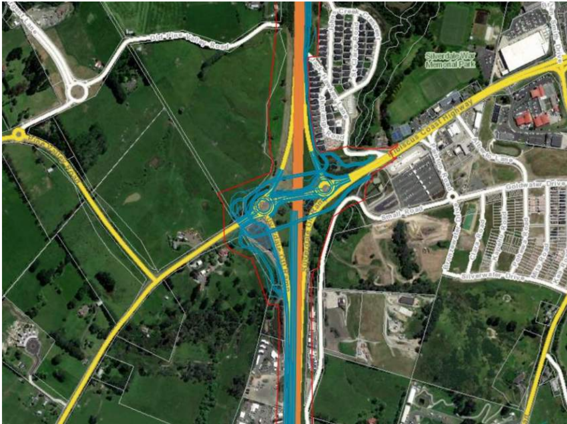
Figure 117: Preferred route for Upgrade to Silverdale Interchange
