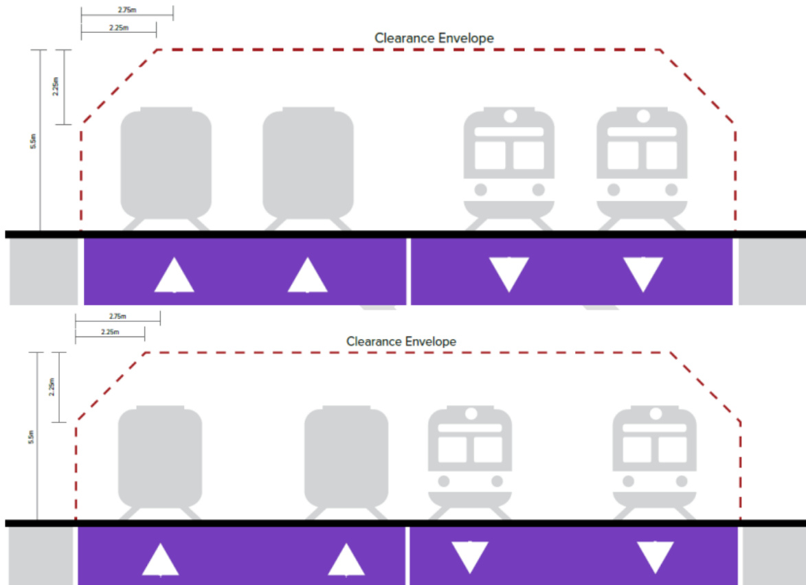
Figure 3-2: General clearance requirements for four-tracking, with two future tracks to one side of existing tracks (top) and a future track to either side of existing tracks (bottom)
