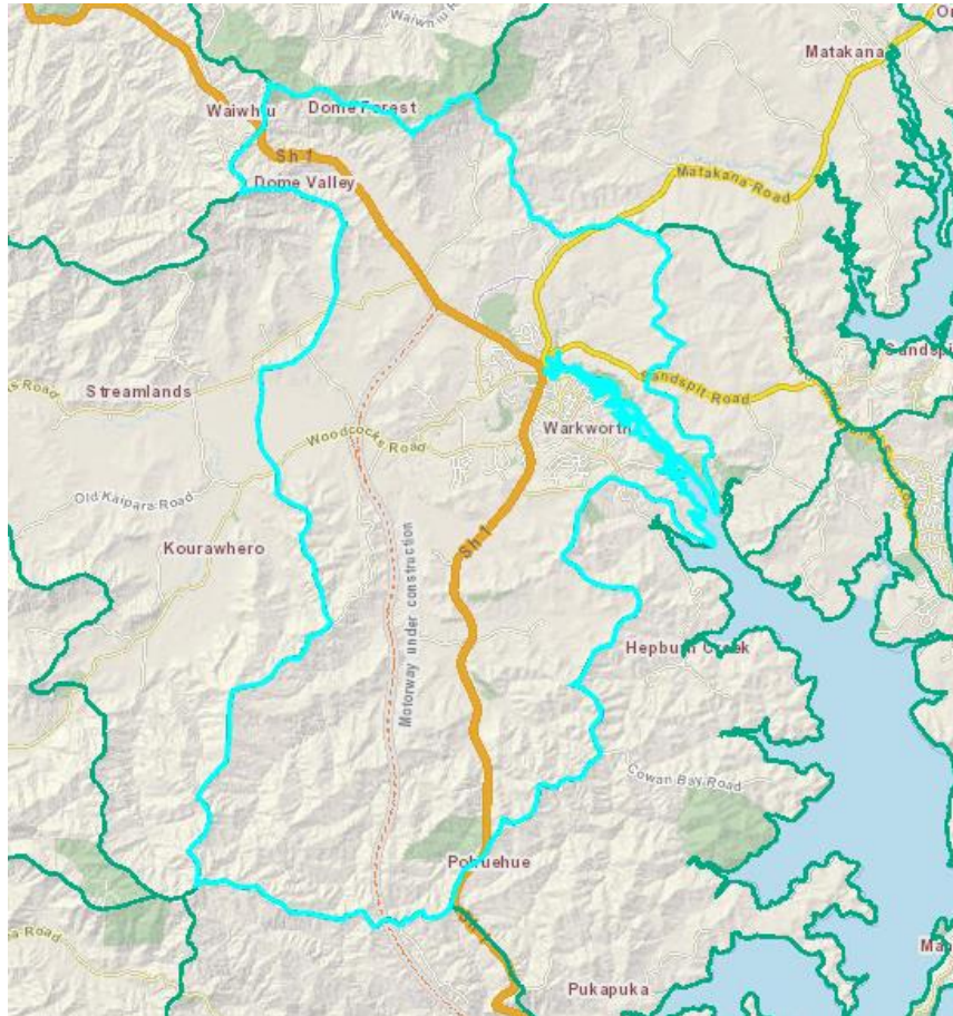
Figure 9.2: Warkworth Stormwater Catchment Boundary outlined in blue
