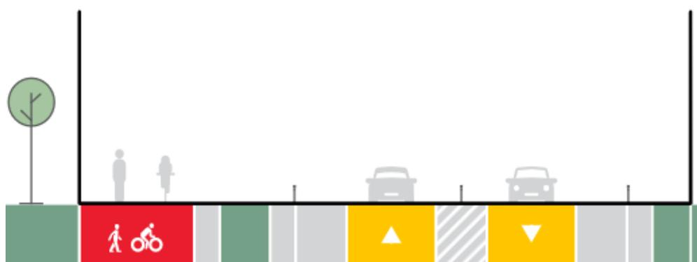
Figure 14-3: Coatesville-Riverhead Highway CFAF cross section outcome S2: Short Road to Riverhead Road Indicative 24m cross section
