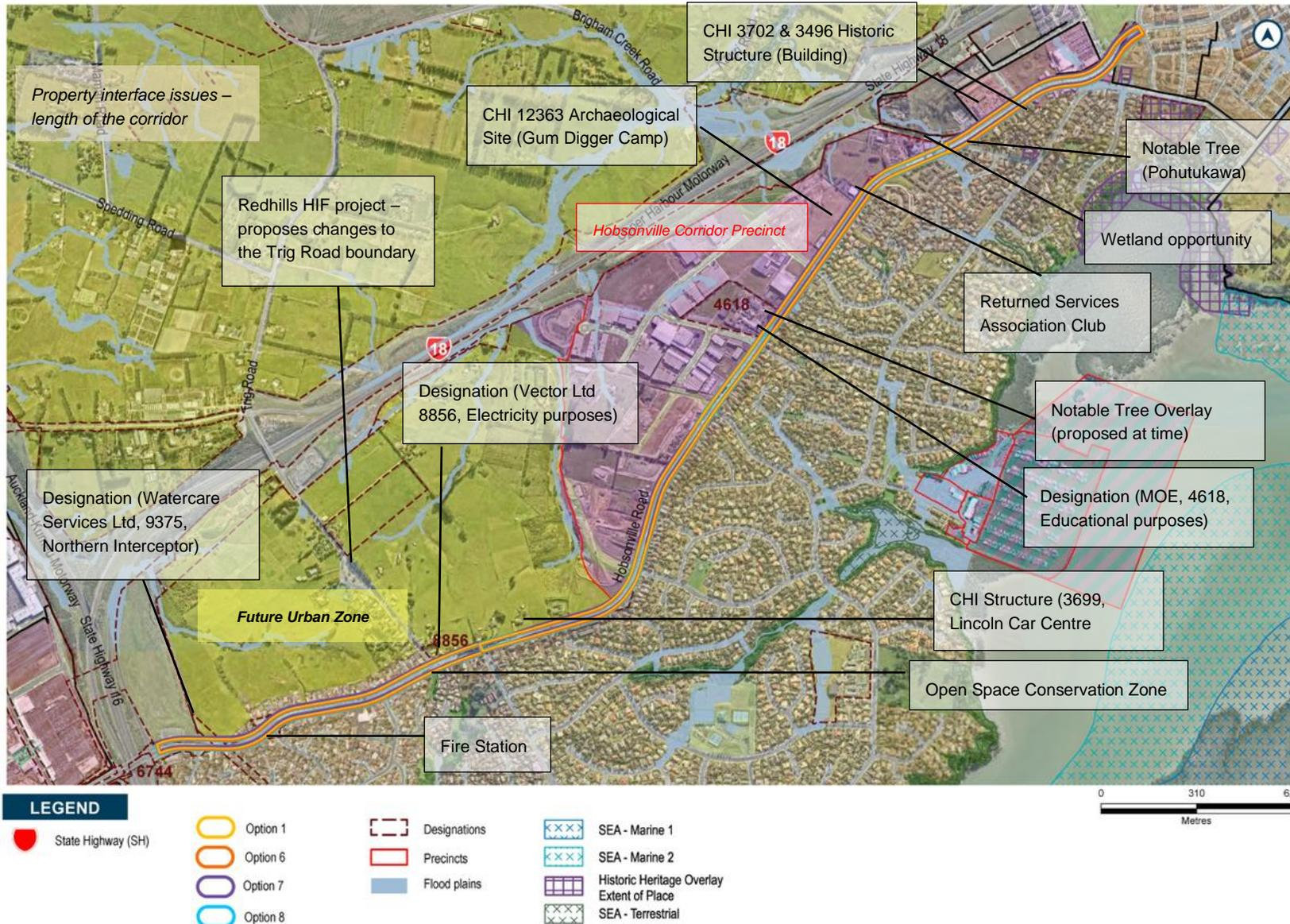
Figure 11-6: Hobsonville Road options and identified constraints
