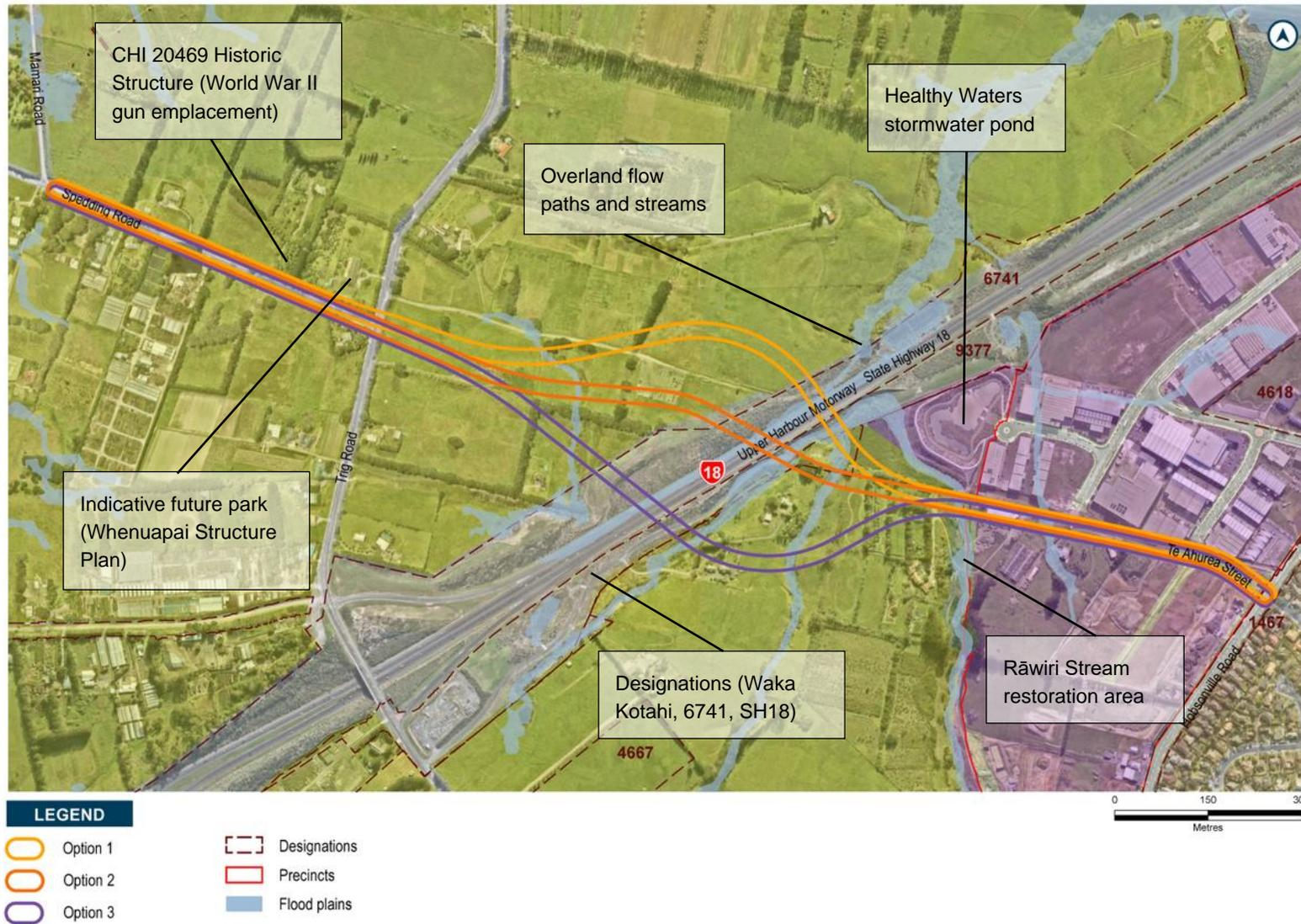
Figure 9-3: Spedding Road East Options and identified constraints
