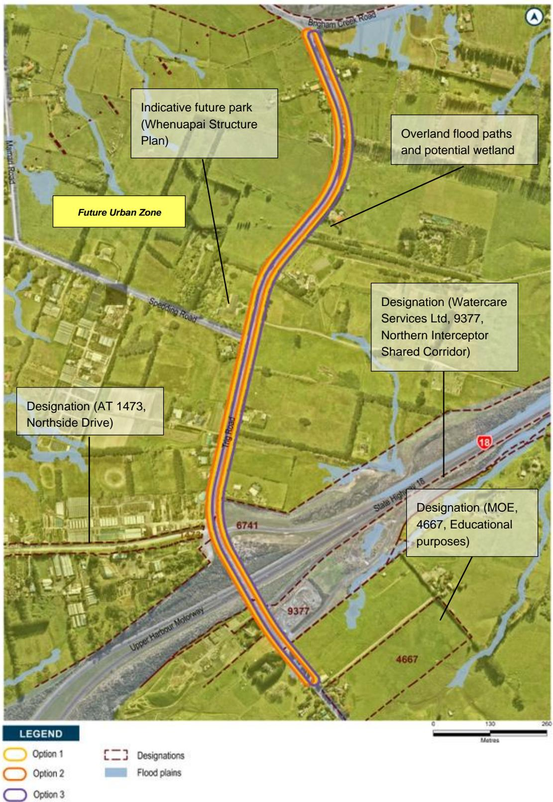
Figure 6-3: Trig Road options and identified constraints
