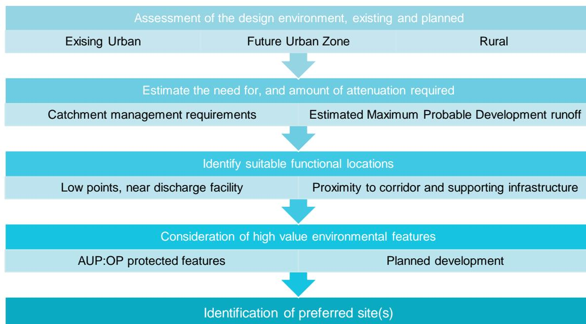
**Figure 4-6: Stormwater infrastructure design and location approach**
