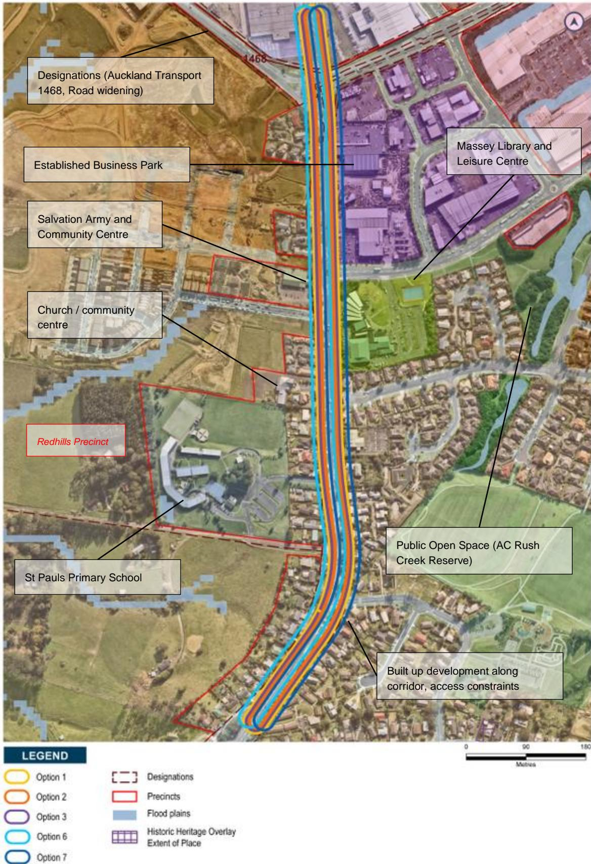
Figure 12-3: Don Buck Road Options and identified constraints
