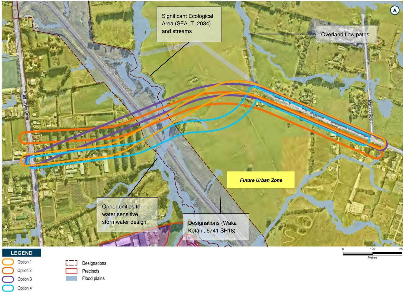
Figure 10-3: Spedding Road West Options and identified constraints
