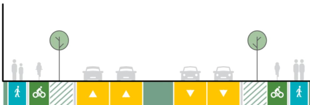
Figure 8-2: CFAF Outcome S1 (BCR interchange to Totara Road segment) Indicative 30m cross section
