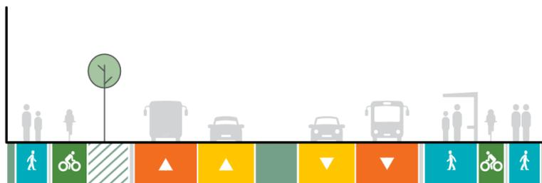
Figure 11-3: CFAF Outcome S2: SH16 Interchange to Luckens Road Indicative 30m cross section
