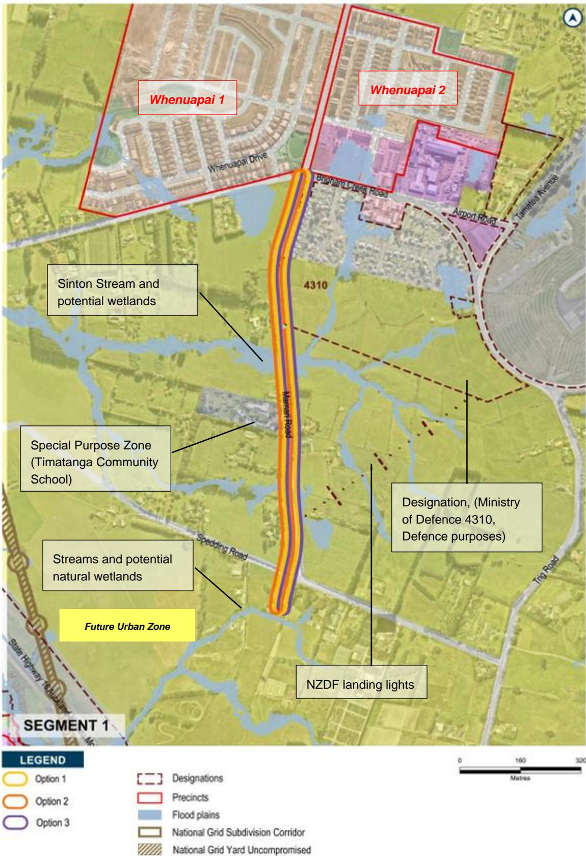
Figure 7-4: Māhari Road Segment 1 options and identified constraints
