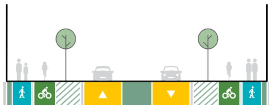
Figure 6-2: CFAF Outcome – Trig Road North indicative 24m cross section
