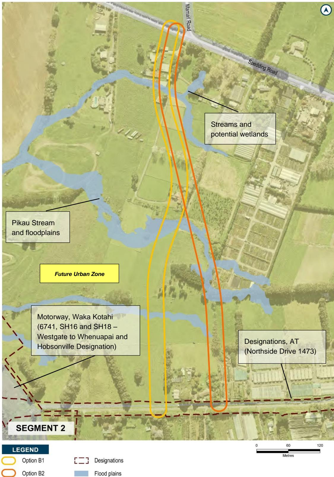
Figure 7-5: Māmari Road Segment 2 options and identified constraints
