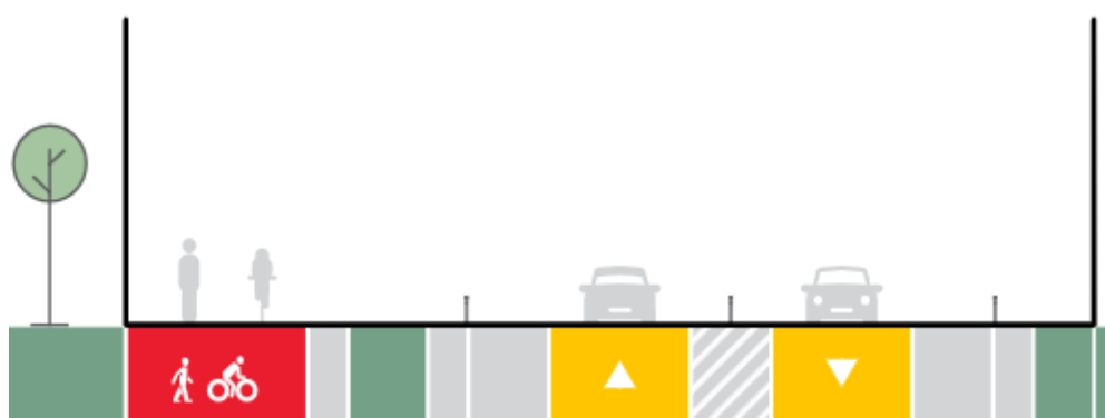
Figure 14-3: Coatesville-Riverhead Highway CFAF cross section outcome S2: Short Road to Riverhead Road Indicative 24m cross section
