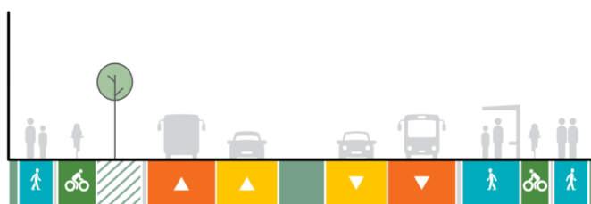
Figure 180: CFAF Outcome - Upgrade and Extension to Bawden Road indicative 30 m cross section
