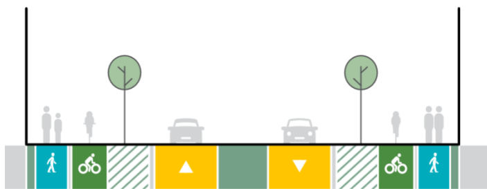
Figure 191: CFAF Outcome - Upgrade to East Coast Road between Silverdale and Ō Mahurangi Penlink indicative 24 m cross section
