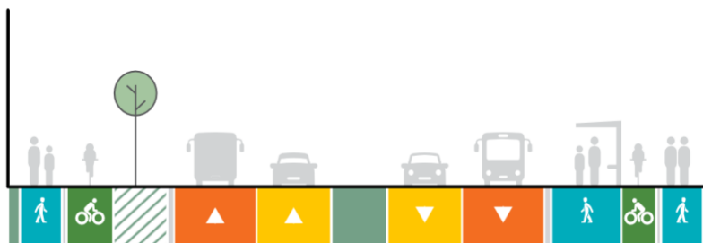
Figure 128: CFAF Outcome - New Connection between Milldale and Grand Drive indicative 30 m cross section
