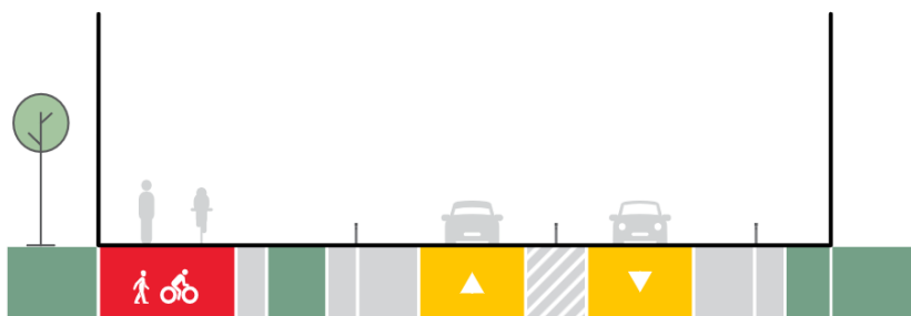
Figure 192: CFAF Outcome - Upgrade to East Coast Road between Silverdale and Ō Mahurangi Penlink indicative 29 m cross section
