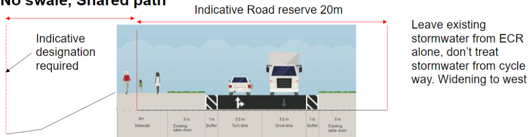
Figure 196: Revised widening options for rural segment 2
