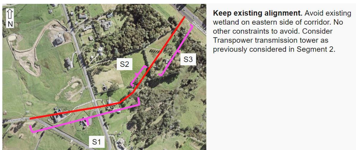
Figure 186: Recommendations for Bawden Road Segment 3
