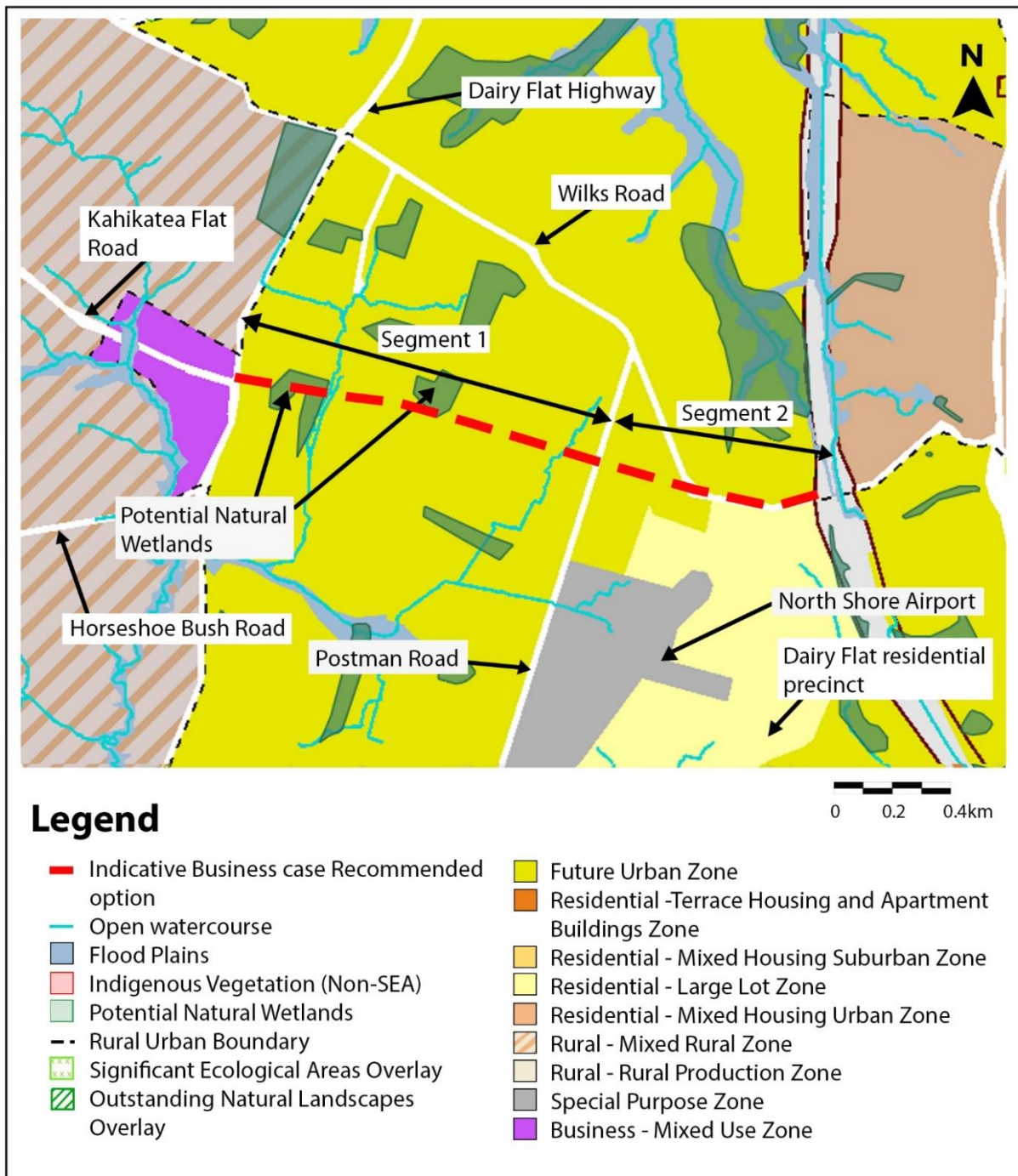
Figure 175: Map of key constraints and features – New Connection between Dairy Flat Highway and Wilks Road
