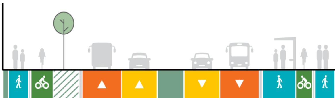
Figure 5-10: Four-lane FTN arterial as proposed for Alfriston Road (section 6 of the Takaanini FTN)
