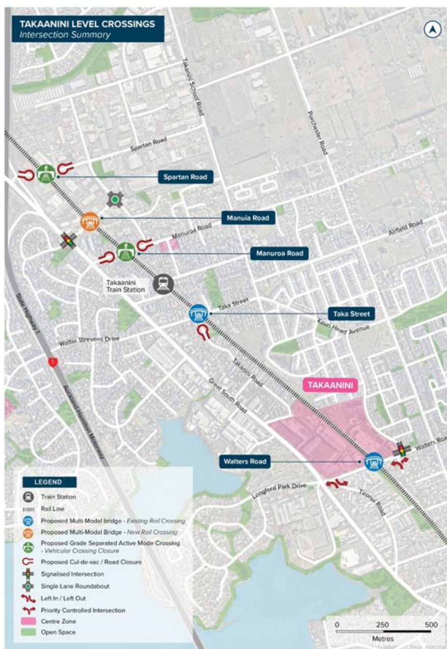
Figure 10-3 - TLC network – indicative intersection forms
