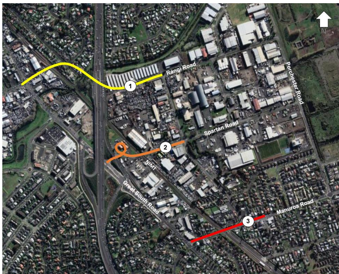
Figure 7-2 - Locations of potential grade-separated crossings at Rangi Road (option 1), Spartan Road (option 2), and Manuroa Road (option 3)
