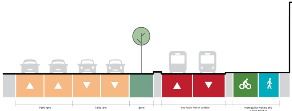
Figure 6: NoR 4a Typical cross section
