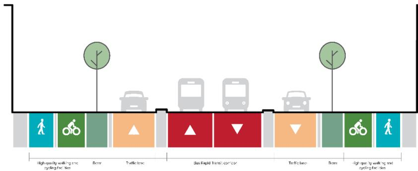
Figure 11: NoR 3 Typical Cross Section (without station)
