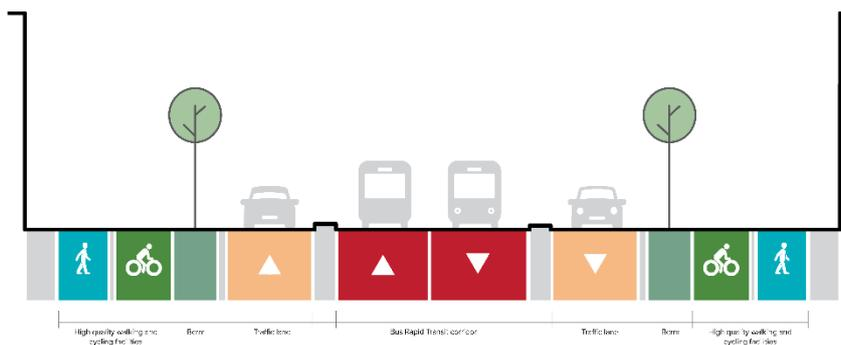
Figure 55: NoR 3 Typical cross section (without BRT station)
