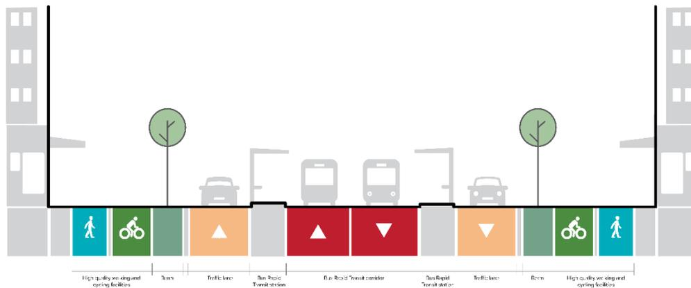
Figure 54: NoR 3 Typical cross section (with BRT station)
