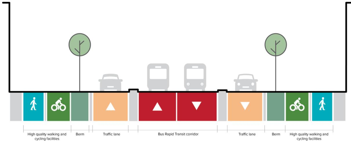
Figure 5: NoR 3 Typical cross section (without BRT station)
