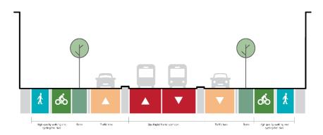
Figure 55: NoR 3 Typical cross section (without BRT station)
