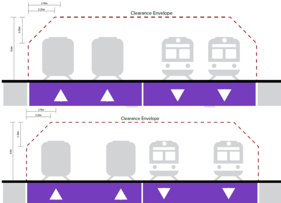
Figure 3-2: General clearance requirements for four-tracking, with two future tracks to one side of existing tracks (top) and a future track to either side of existing tracks (bottom)
