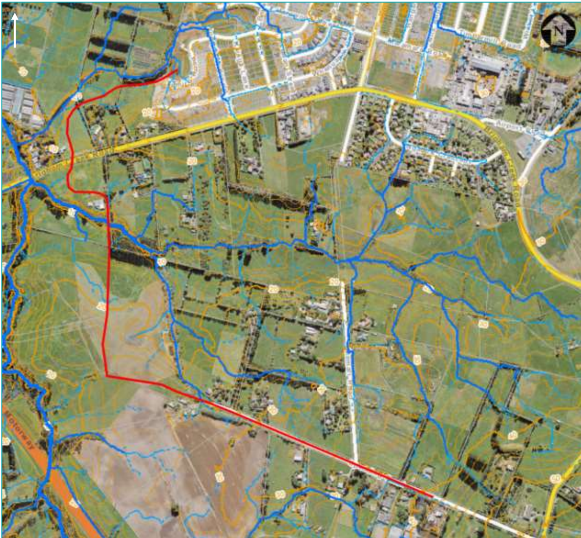
Figure 6. Contour information with overland flow paths – approximate site alignment shown as red line (Auckland Council Geomaps)
