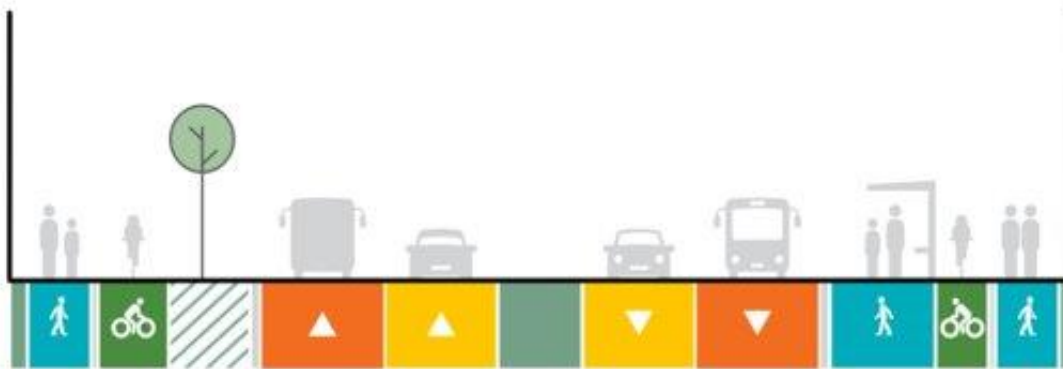
Figure 1-3: Indicative future Māmari Road corridor design
