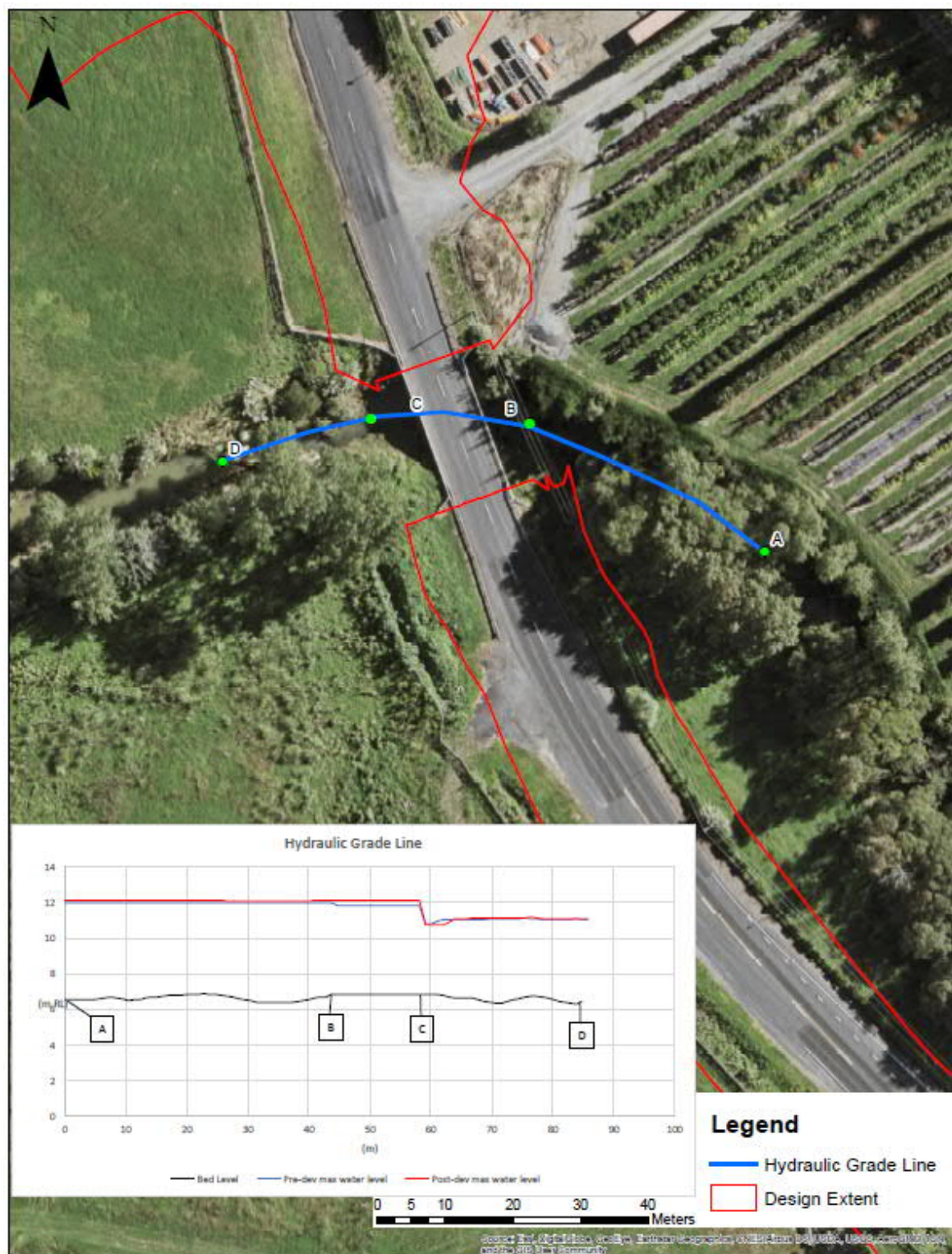
Figure 9-10: Hydraulic grade line, 100 year ARI at Ōpāheke Road and Ōtūwairoa Stream crossing
