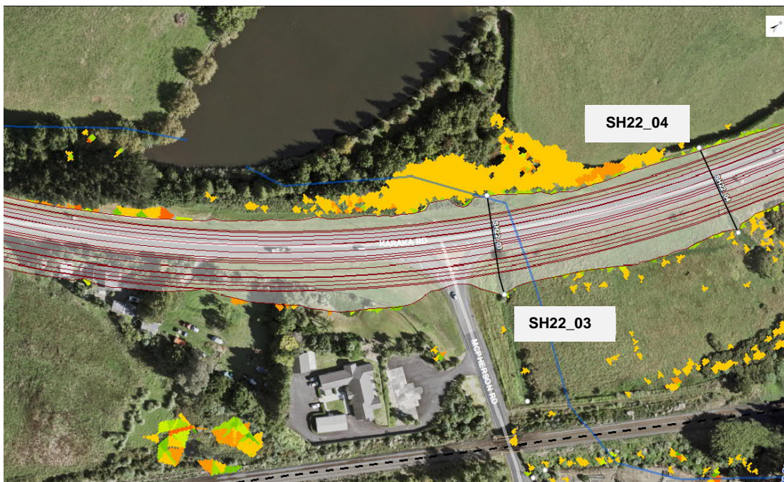
Figure 5-6: 10 Year difference map for post- minus pre-project development at SH22 and existing crossing at chainage 2320 (SH22-03) and at chainage 2200 (SH22-04)
