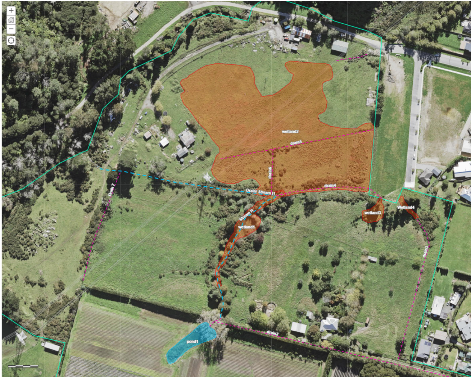
Figure 5. The most northern portion of the PPC site (turquoise boundary, showing Stream I1 (dotted blue line), NPS-FM qualifying natural inland wetlands (red shaded polygons) and constructed drains (purple dotted lines). The constructed pond for horticultural water supply is indicated as a blue polygon.
