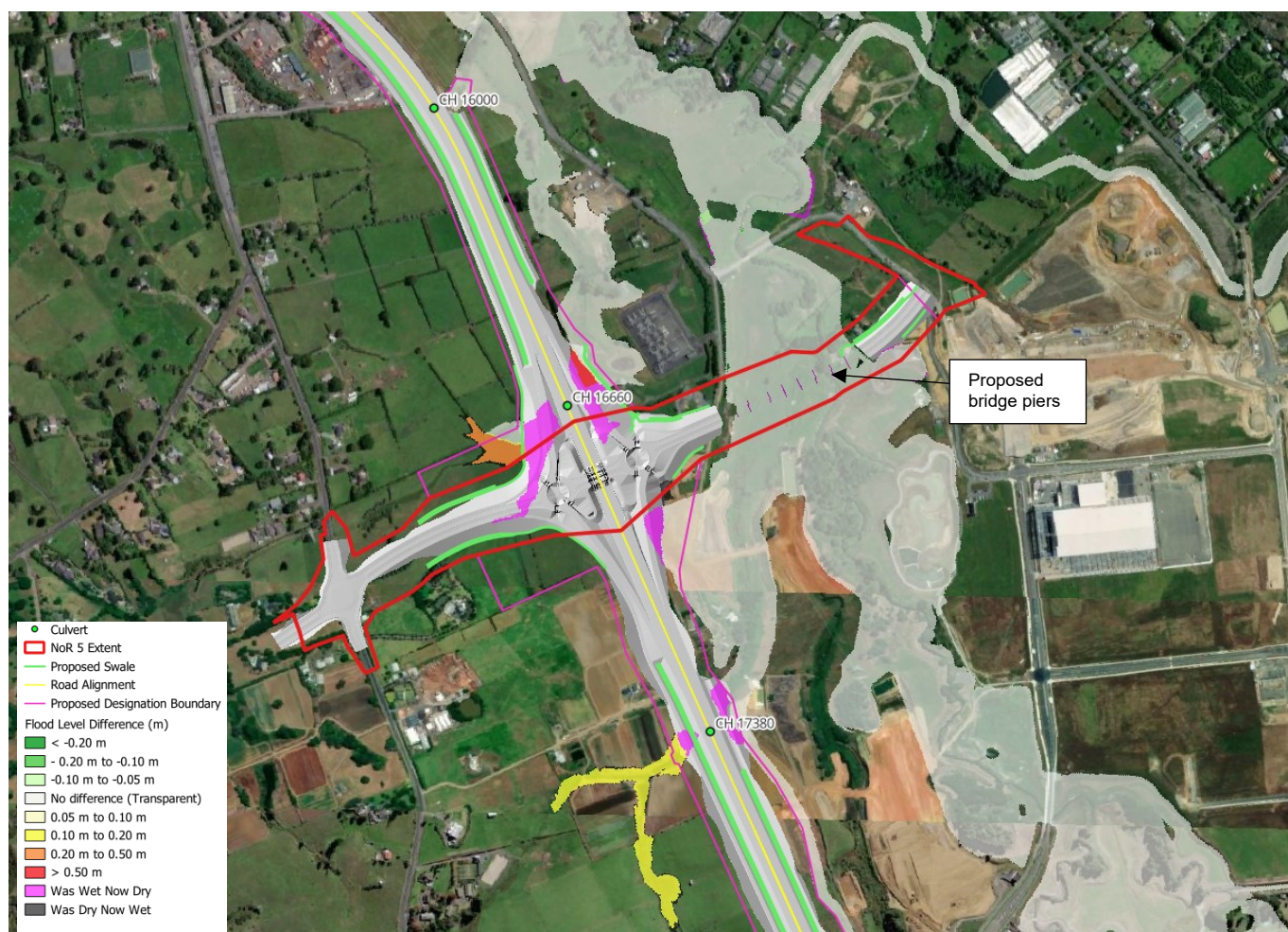
Figure 10-4 Flood impact (post-development vs pre-development) for the 1% AEP event with climate change – NoR 5
