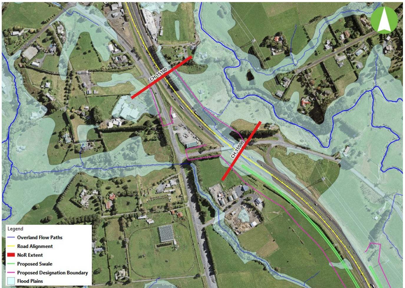
Figure 6-3 Proposed swale within NoR 1 project boundary
