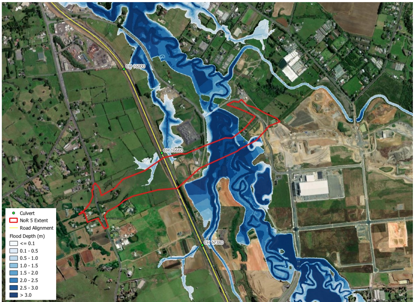
Figure 10-2 Flood extent 1% AEP event with climate change – Baseline scenario
