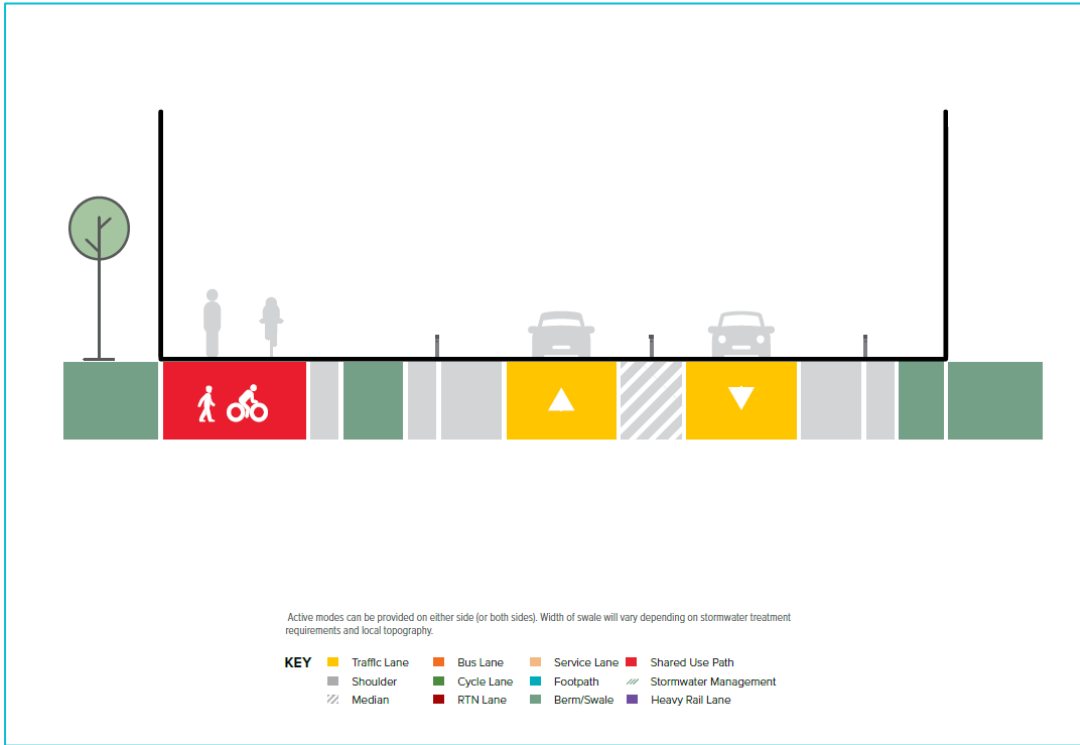
Figure 6-4: Generic 24m wide cross section is proposed with two lanes for general traffic and active transport facilities on one side of the corridor.
