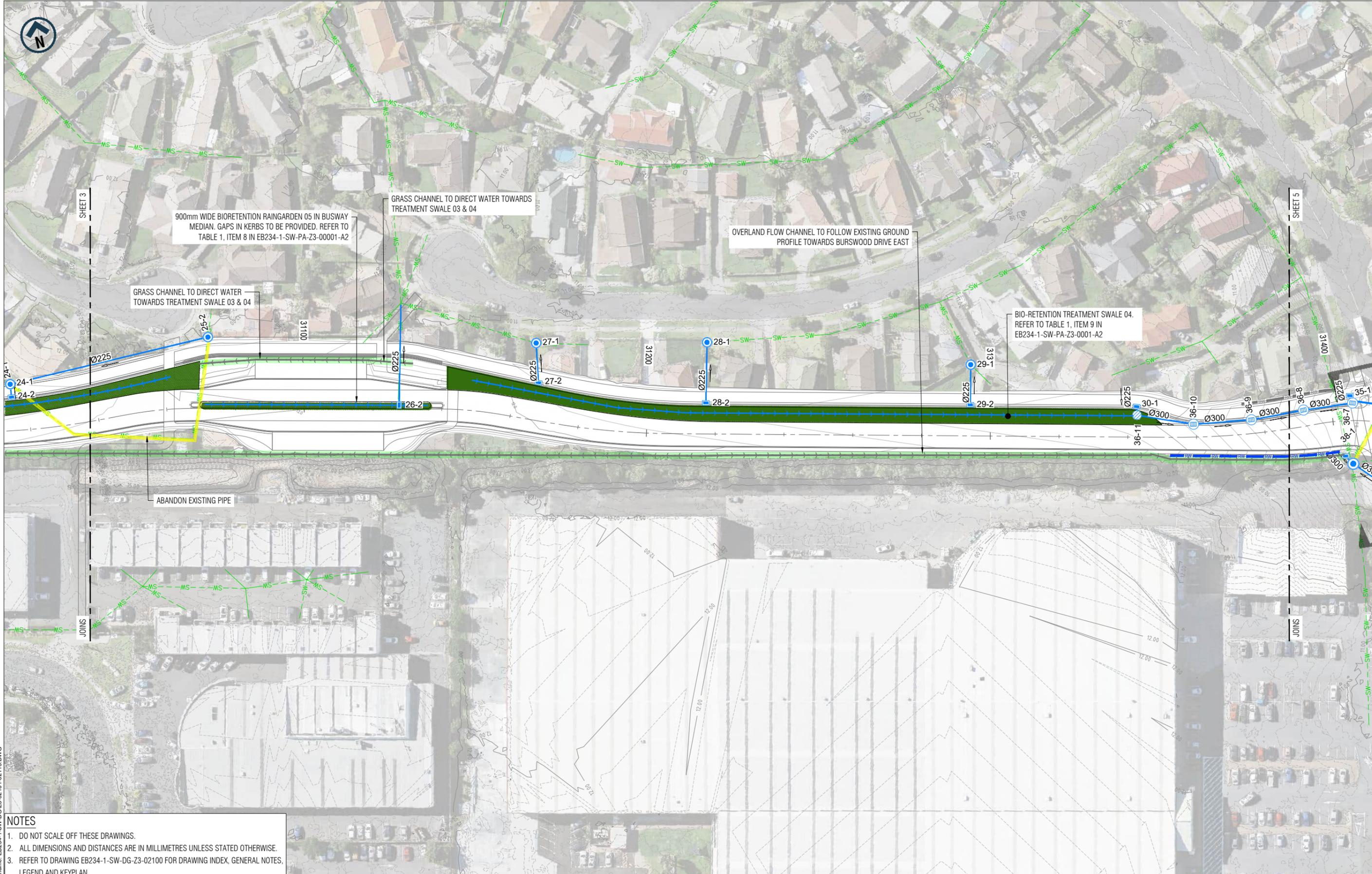
900mm WIDE BIORETENTION RAINGARDEN 05 IN BUSWAY MEDIAN. GAPS IN KERBS TO BE PROVIDED. REFER TO TABLE 1, ITEM 8 IN EB234-1-SW-PA-Z3-00001-A2
