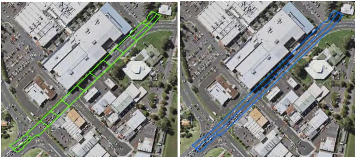
Figure 4: Flyover sub-catchments loaded to downpipes (green) and flyover sub-catchment to be loaded to the pipe network to the west in the detailed design stage (blue).
