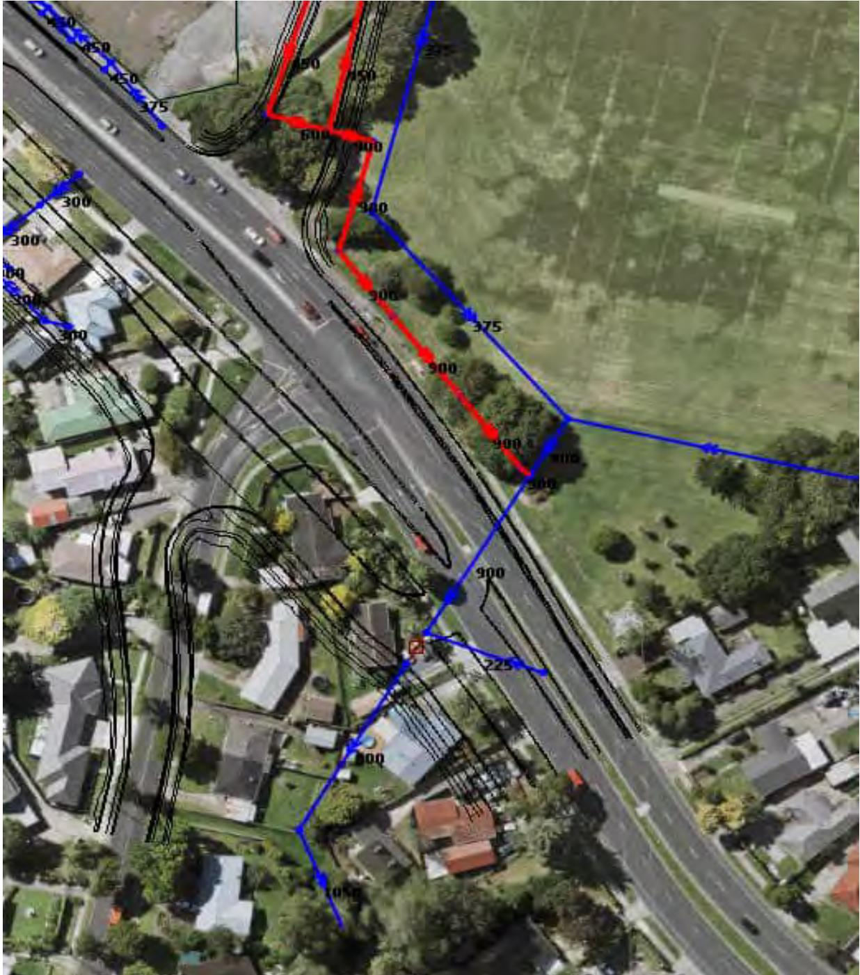
Figure 10: WRR design network highlighted in red connecting to the existing pipe network shown in blue.
