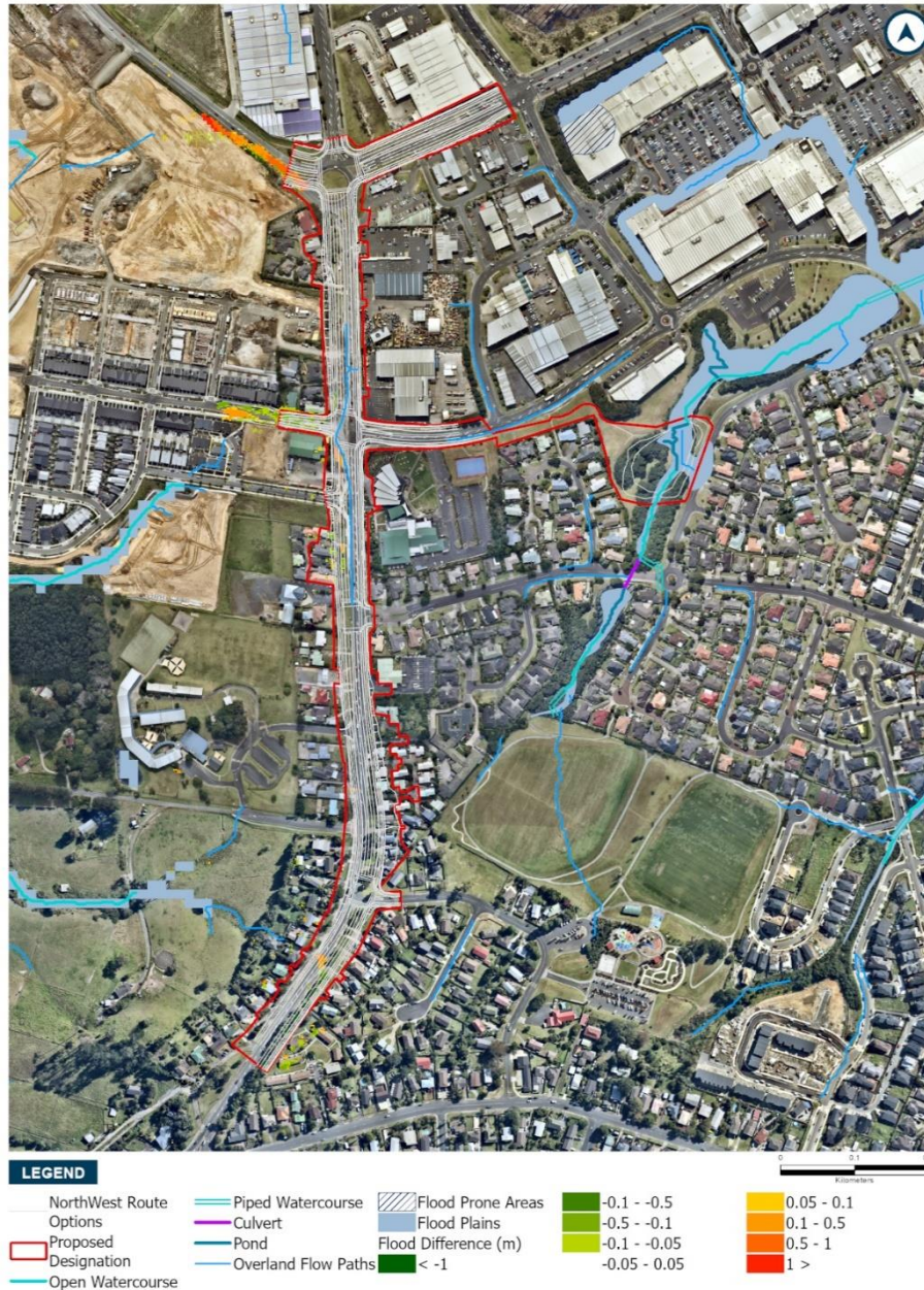
Figure 9-1: 100 year ARI flood difference map for Don Buck Road
