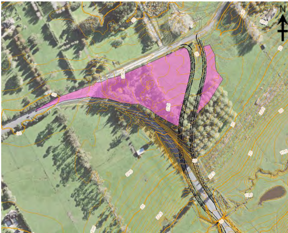
Figure 5.6: Catchment Draining to Proposed Channel
