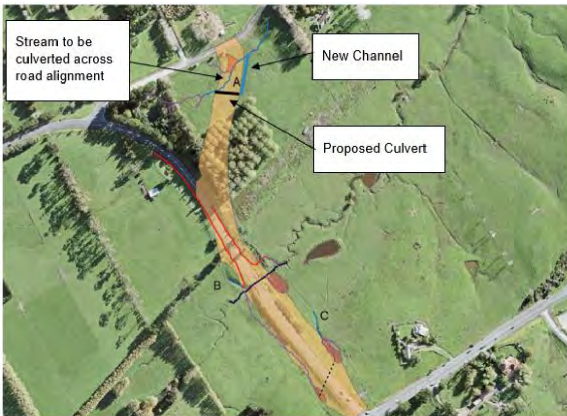
Figure 5.5: Intermittent Stream Alignment
