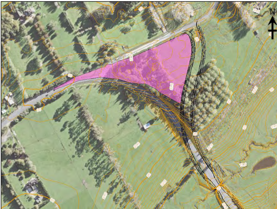
Figure 5.4: Catchment to Proposed New Culvert at Road Chainage 550m
