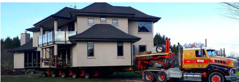
Low loader house removal truck and trailer unit
