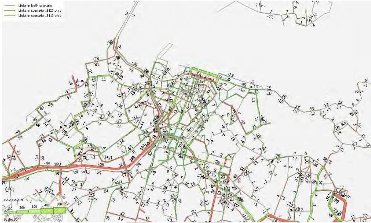
Figure 7-3- Comparison of Path Based Assignment vs Standard Parallel Assignment – AM Peak – red bars show more traffic in path based test, green bars show less traffic
