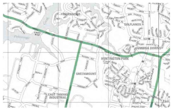
Figure 31: Over-dimensional vehicle routes
