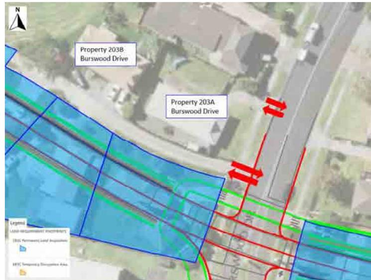
**Figure 68: Property accesses (red arrows) to be maintained during construction at 203 Burswood Dr**
