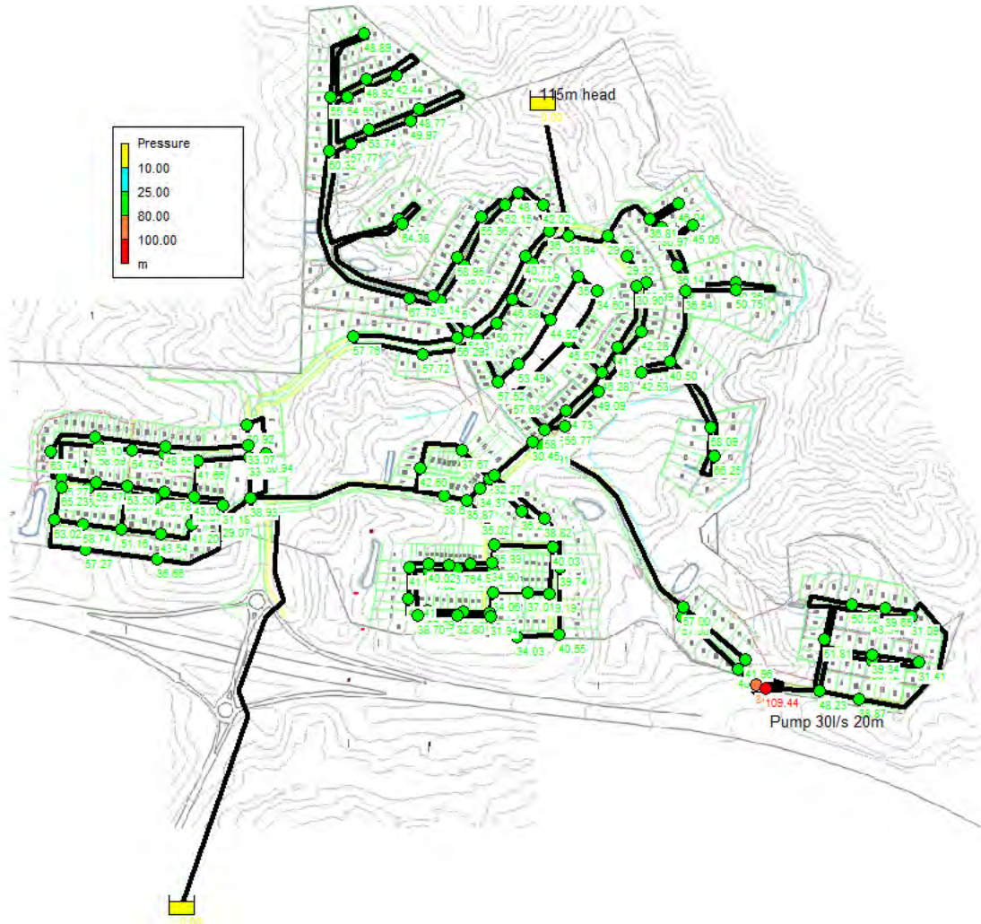
Figure 4 Scenario 2 Pressure at Nodes
