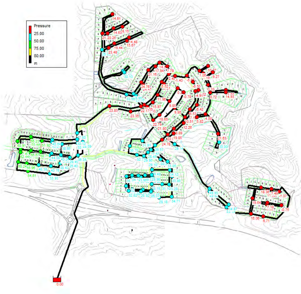
Figure 6 Scenario 3 Pressure at Nodes
