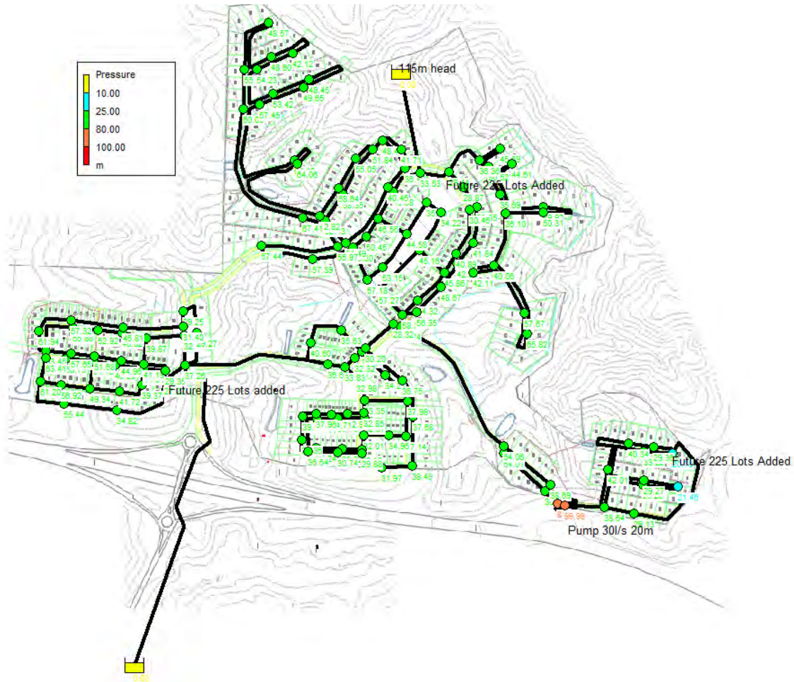
Figure 8 Scenario 4 Pressure at Nodes
