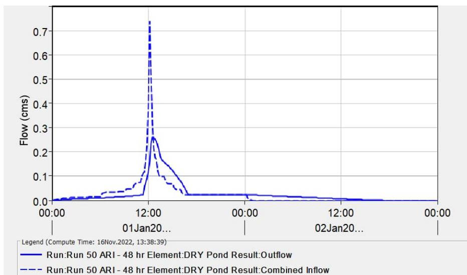
**Figure A3-2. Dry Pond – 2% AEP (50yr ARI) Inflow and Outflow Graph (Post-Development)**
