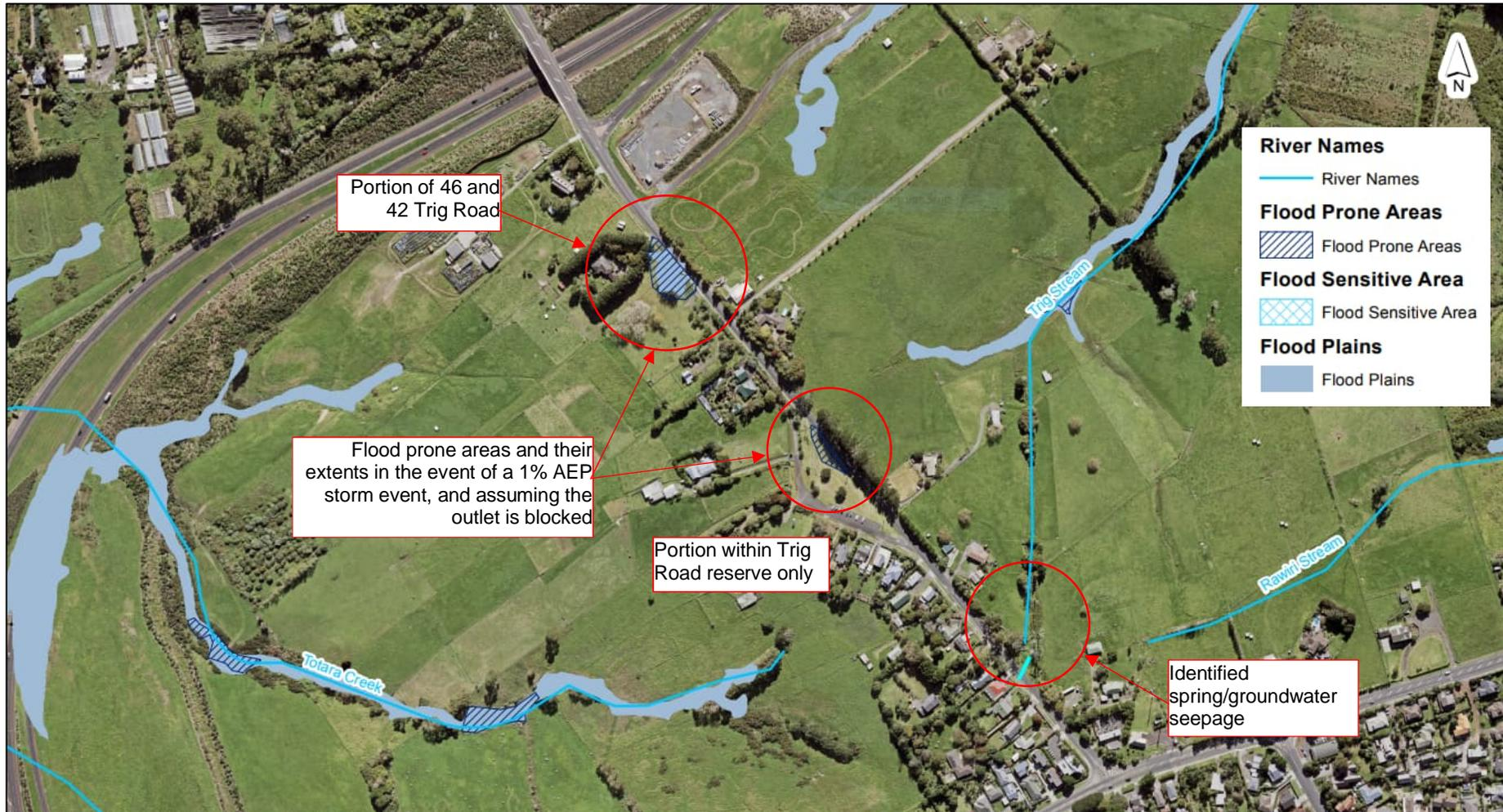
Figure 8: Existing flood plain and flood prone areas along Trig Road (AC – Geomaps 2022)
