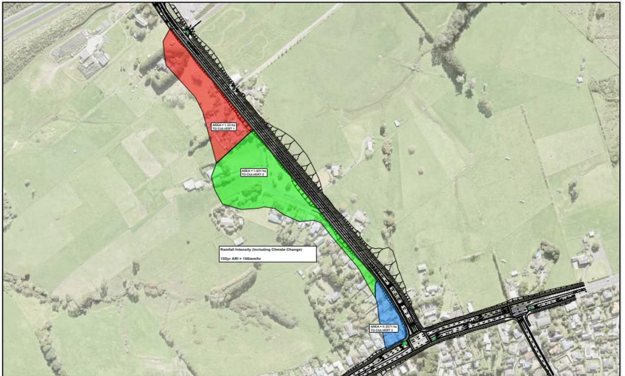
Figure 10: Post-development catchments for culvert/pipe flows
