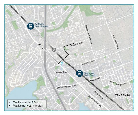
Figure 56: Walk diversion route to a location in the north if no active mode connection is provided at Spartan Road
