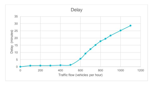
Figure 19: Delay caused by barrier downtime in the future network
