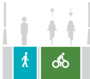
Figure 46: Typical cross section for active mode bridges
