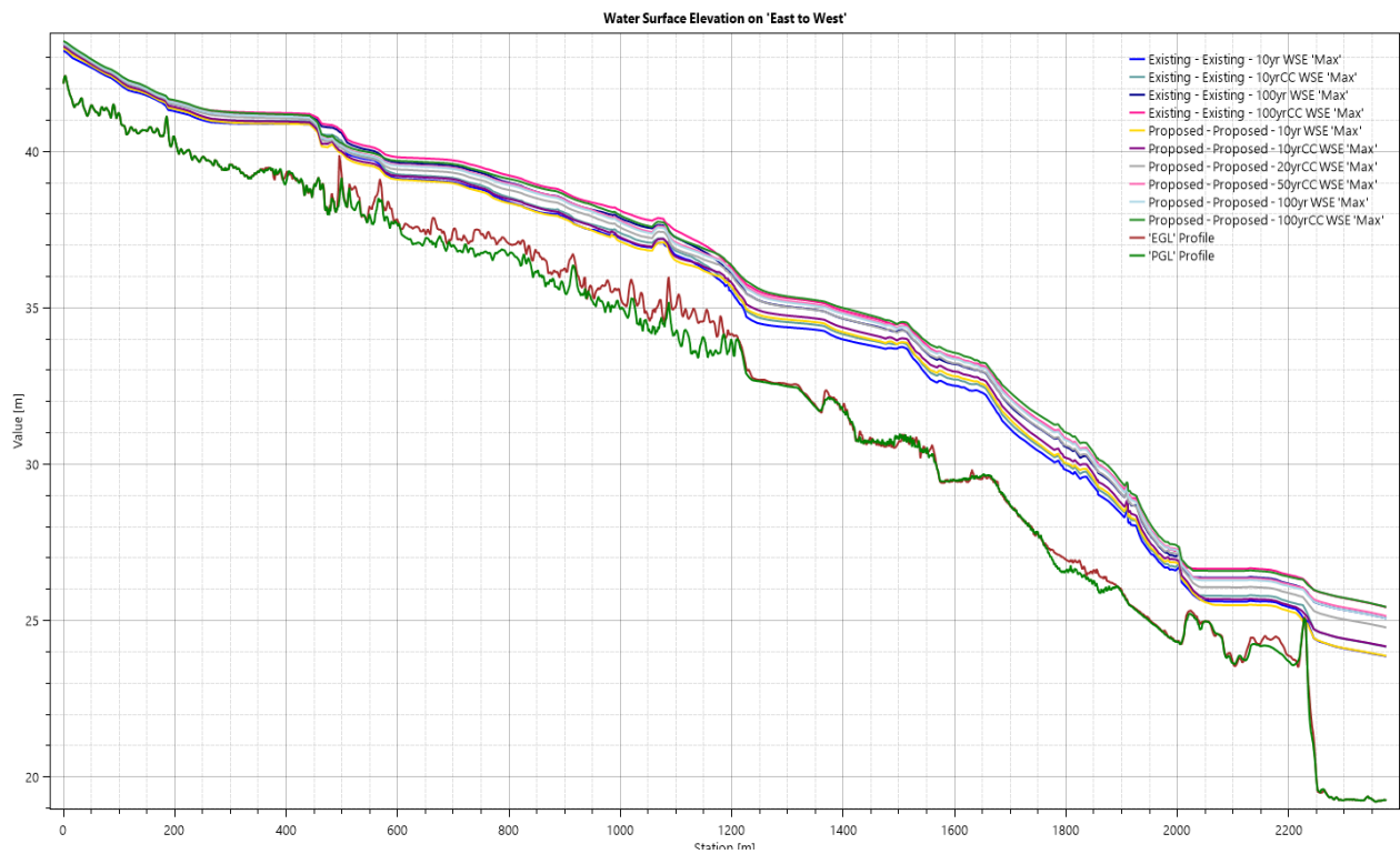
Figure 3.4 – HGL– Main east to west stream (NZVD)
