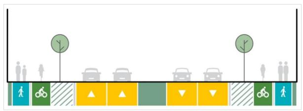
Figure 10-1: Access Road Typical Cross Sections
