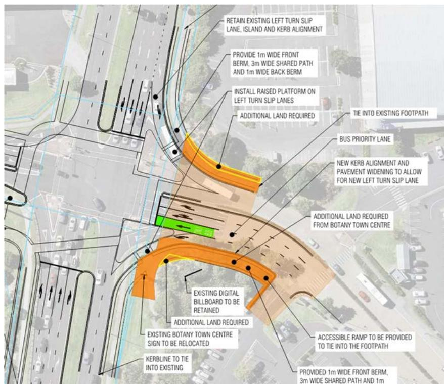
Figure 6-2 Proposed intersection improvement works of Te Irirangi Drive and Town Centre Drive.
