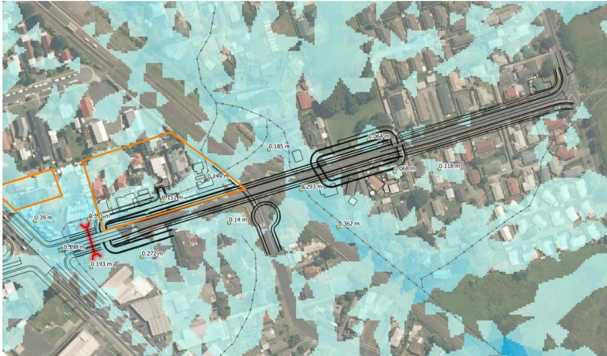
**Figure 4: Auckland Council ICM model Flood Results (1% AEP+CC flood depths)**
