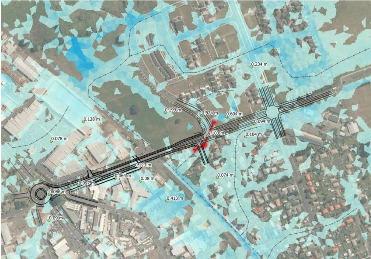
**Figure 5: Auckland Council ICM model Flood Results (1% AEP+CC flood depths)**
