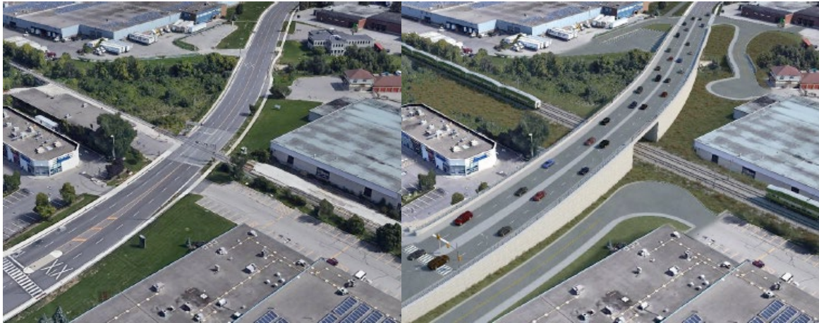
Figure 5-3: Progress Avenue crossing before (left) and after (right) grade separation
