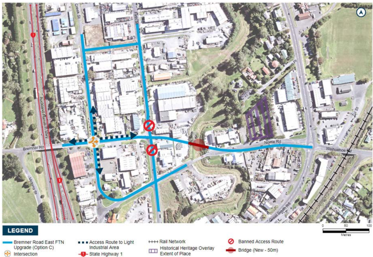
Figure 15-12: Option C – short bridge, Firth Street rerouted
