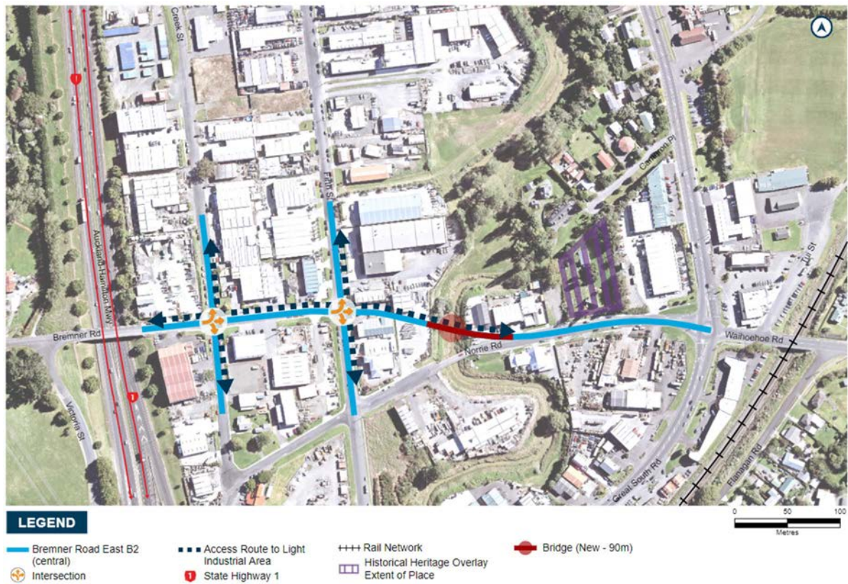
Figure 15-11: Option B2 – Medium bridge, intersections at Firth and Creek Street
