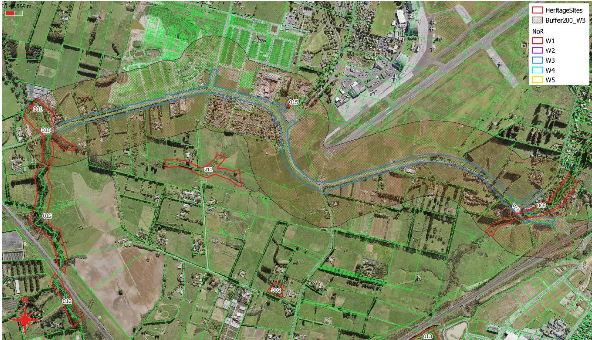
Figure 15: NoR W3 corridor in relation to the 200 m buffer and heritage features: shell midden 001, notable tree 015, high risk area 010 (Totara Creek crossing) and 009 (Waiarohia Stream crossing).
