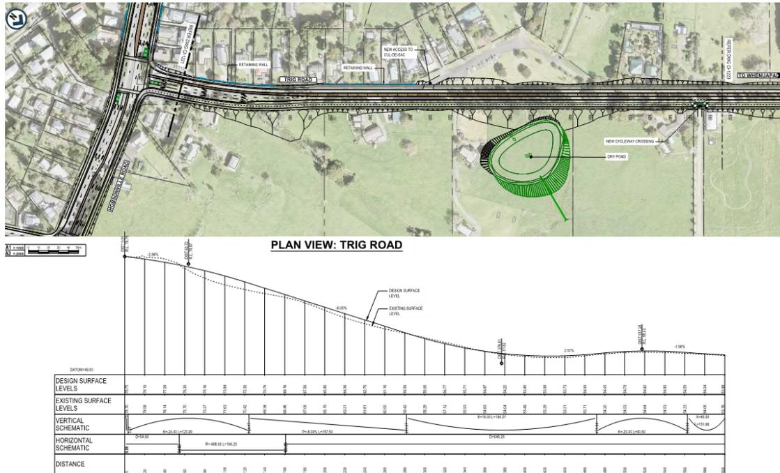
Figure 1 - Trig Road Proposed Concept Design
