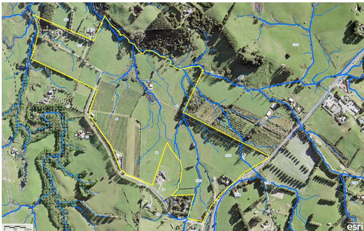
Figure 1. A map of the Warkworth South Plan Change site (yellow polygon) showing predicted overland flow paths (dark blue lines) and Terrestrial Significant Ecological Areas (SEA-T; green crosses) from Auckland Council's GIS viewer.
