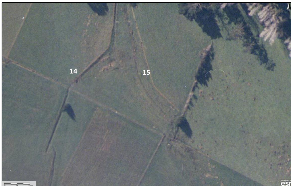
Figure 6. Historical aerial image from 2001, showing the constructed western drain (14) and the potentially modified eastern stream (15). The wetland vegetation growing throughout the area currently, was not present in 2001. Image from Auckland Council's Geomaps.
