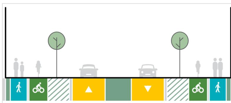
Figure 8-1: SH16 Main Road Upgrade Typical Cross Section
