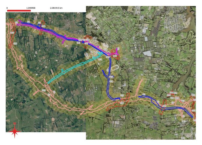
Figure 4-6: NoRs corridors (S1 - S4 in various colours) with 200m buffer zones (hatched areas surrounding NoR corridors), all heritage sites (numbered 027 - 034) and high risk areas (numbered 035 -040) within these buffer zones.
