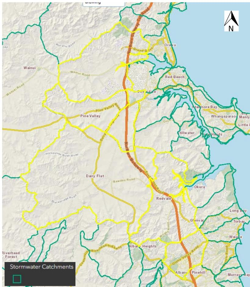
Figure 4-1: North Project stormwater catchments (relevant catchments indicated in yellow)
