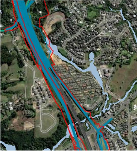
**Figure 6-1: NOR 1 and 4 flooding impacts in Lucas Creek for the 1% AEP future base case scenario**
