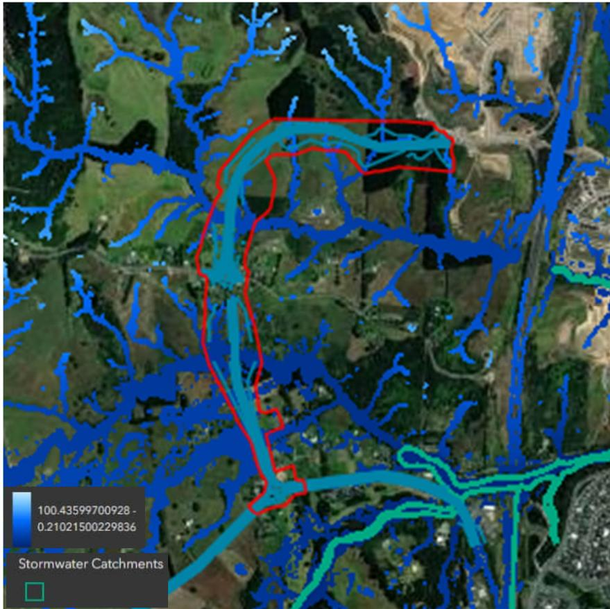
**Figure 11-2: NOR6 Milldale to Grand Drive connection predicted future 1% AEP base case flood extents**
