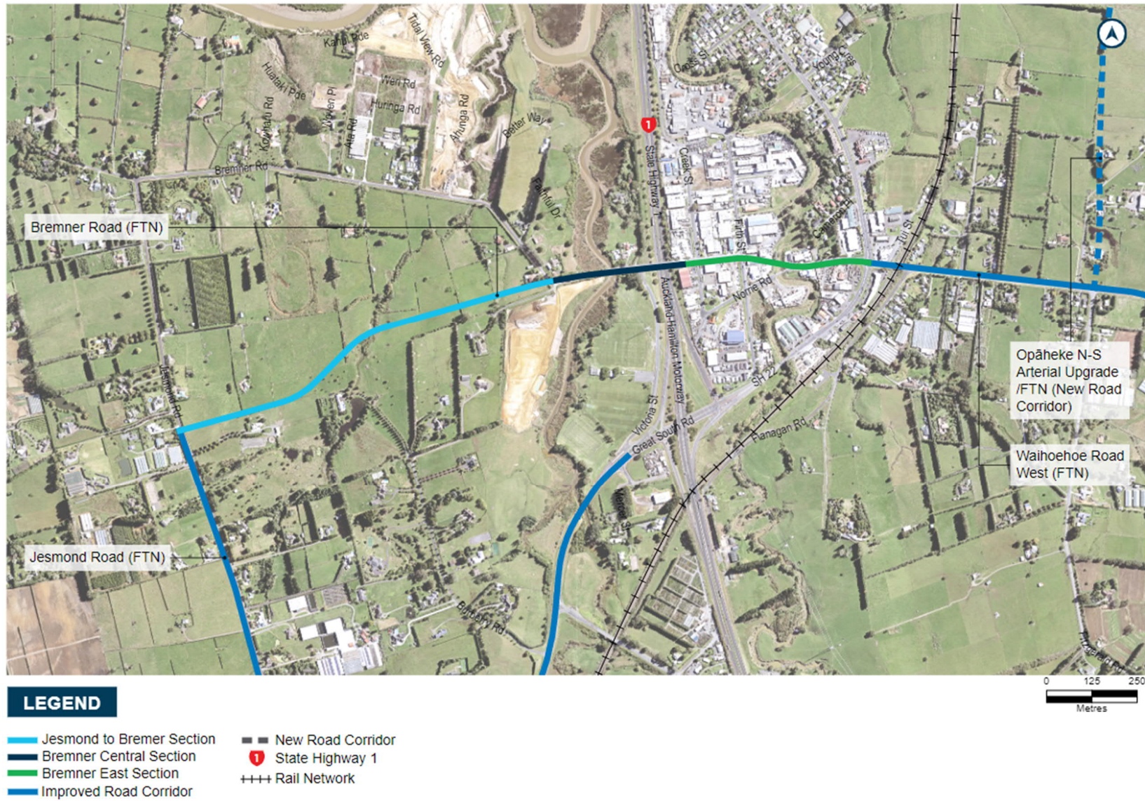
Figure 11-7 Bremner Road FTN Upgrade Assessment Sections
