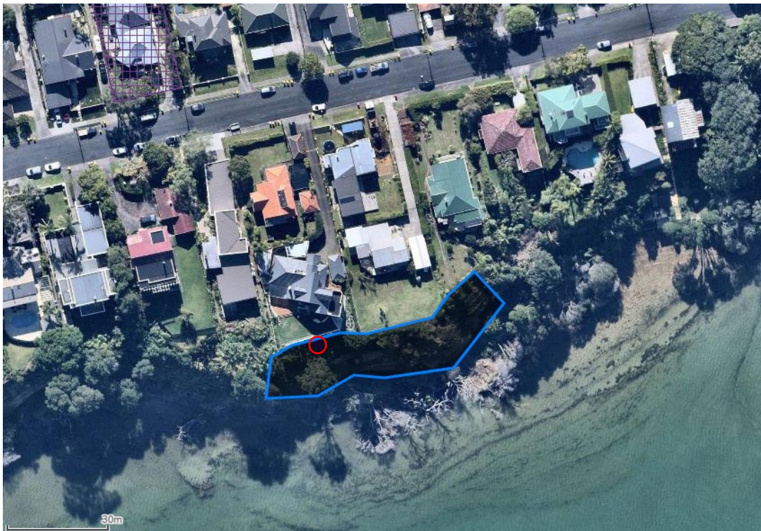
Figure 5: estimated extent of slip at rear of 29 to 35 Norwood Road, overlaid on 2024 aerial imagery. Fallen trees and debris is visible at the toe of the cliff. Historic Heritage place dot for Midden R11_970 is circled in red (Auckland Council GeoMaps).
