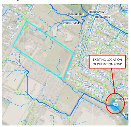
FIGURE 6: Existing Location of Wet Detention Pond.
