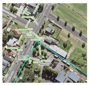
FIGURE 2: Existing Stormwater Network, Auckland Geomaps.
