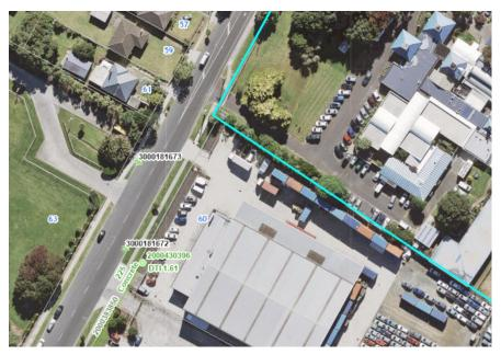
FIGURE 4: Existing Public Stormwater Drainage (60 Westney Rd)
