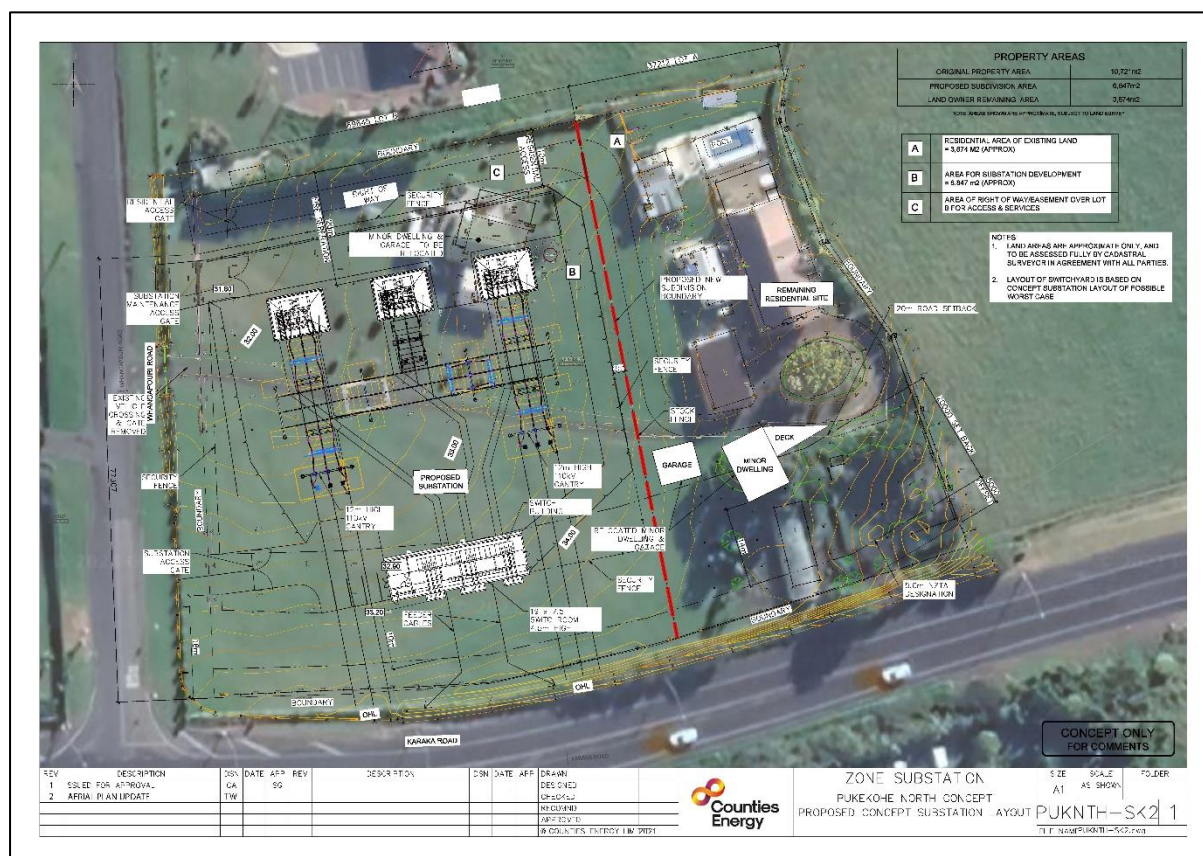
Figure 11 Concept substation layout provided by Counties Energy.
