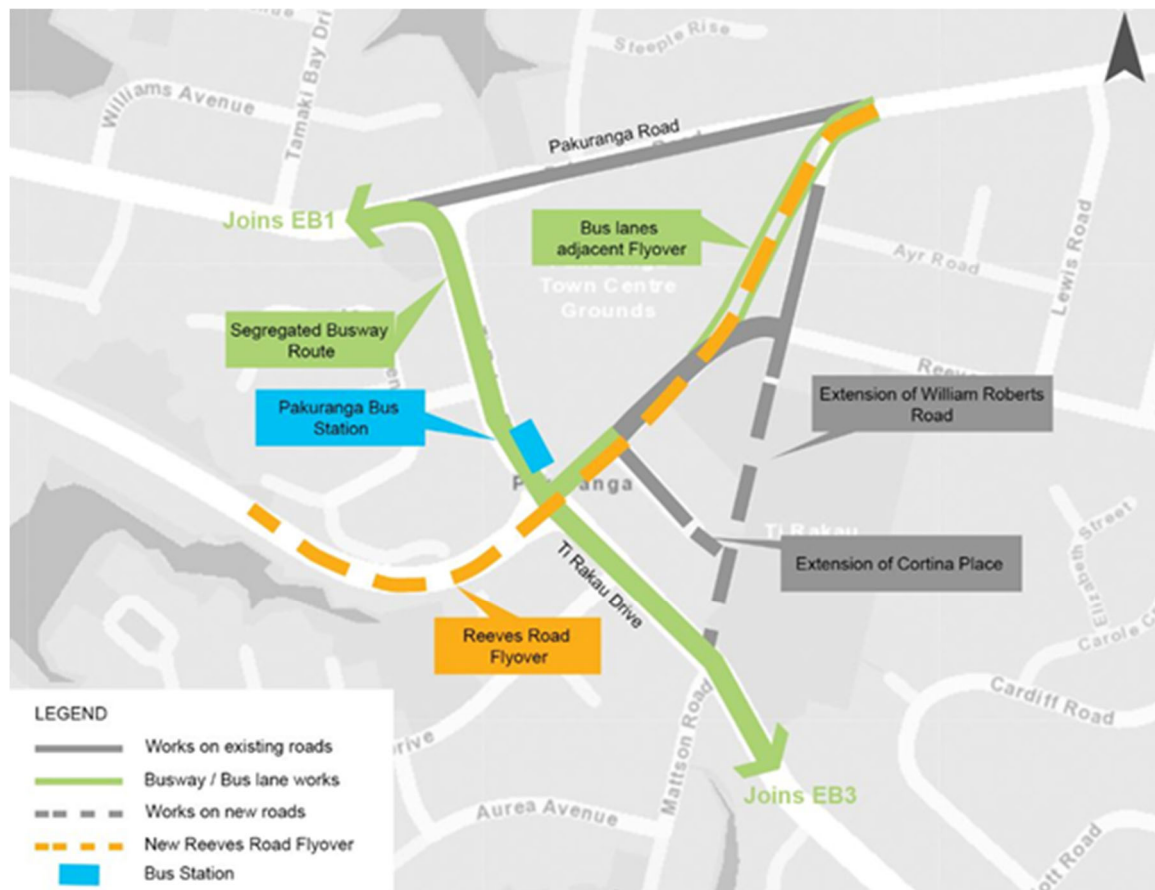
Figure 1 Overview of EB2
