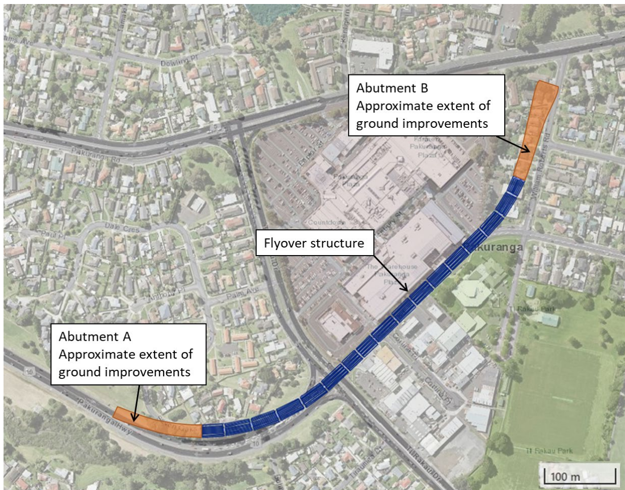
Figure 2. Indicative location of ground improvements required for Abutments A and B, Reeves Road Flyover.
